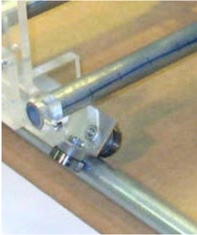
Figure 1 – Rolling Bearings on a Track
